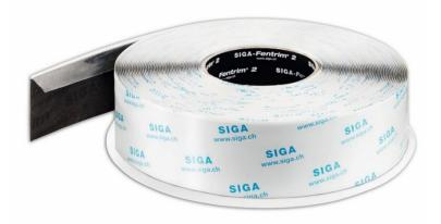
The black colored, single-sided high-performance adhesive tape Fentrim IS 2 is the optimal solution for permanent airtight and driving-rain proof sealing of window and door frames in solid construction on the exterior. According to the rule "less permeable on the inside than on the outside", the white colored window joint tape Fentrim IS 20 perfectly supplements Fentrim IS 2.
